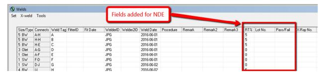
The RT% column is just for information and is not editable. It shows the percent RT required for each weld according to the spec. The Lot No. column is normally filled in by the program. The Test/Pass/Fail column is filled in by the user, by entering the letter T, P or F. The existing column INSP1 is used to store the X-Ray number.
